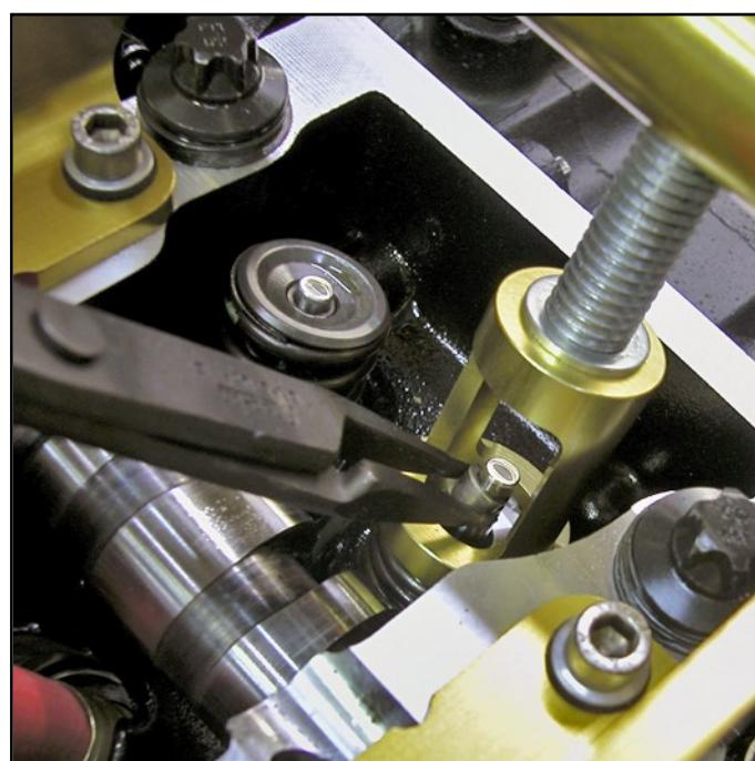
Loosen compression bolt completely and rotate compression rod to allow access to valve. Thoroughly inspect valve spring assembly to ensure cotters are seated properly. **CAUTION: An improperly locked valve spring will cause engine damage.**
