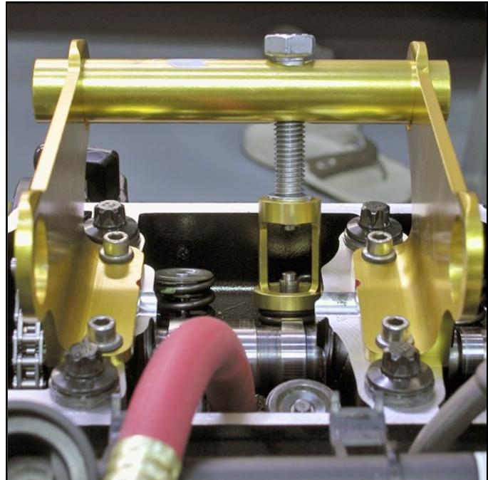
Tighten compression bolt until compression cup seats on valve spring retainer. Check alignment.
