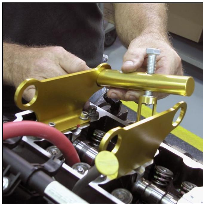
Tighten compression bolt enough to expose valve spring retainer cotters.
