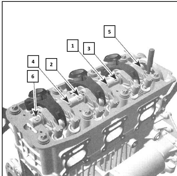
Install spark plug tubes.
