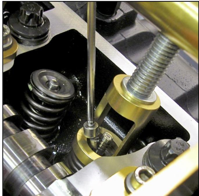
Loosen compression bolt completely. Rotate compression rod to allow access to valve.
