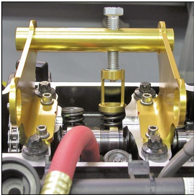
Remove valve spring retainer cotters (2 per valve).
