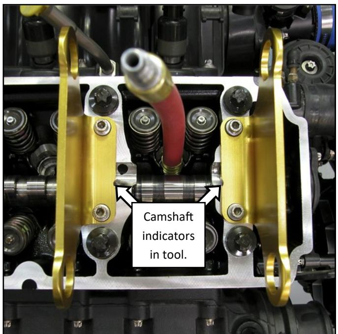
Install supplied airline into spark plug receiver for cylinder being serviced. Using a metered airline, pressurize cylinder to 80psi maximum. **NOTE: When pressurizing cylinder cam chain guide may rise out of cylinder head. Simply hold in place or press back into place.**
