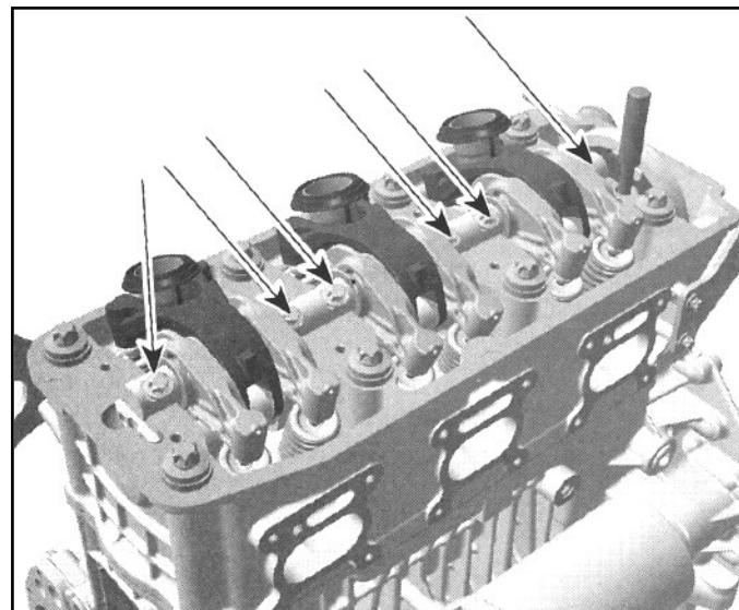
Install compression rod supports onto cylinder head using supplied hardware making sure red indicators are aligned with camshaft.
